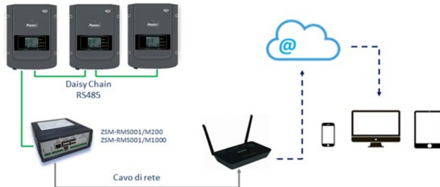
Figure 53 – Diagram showing the operation of the ZSM-RMS001/M200 / ZSM-RMS001/M1000 datalogger
