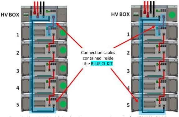
Example of an HV BOX with Amphenol connectors and batteries with Weco connectors
