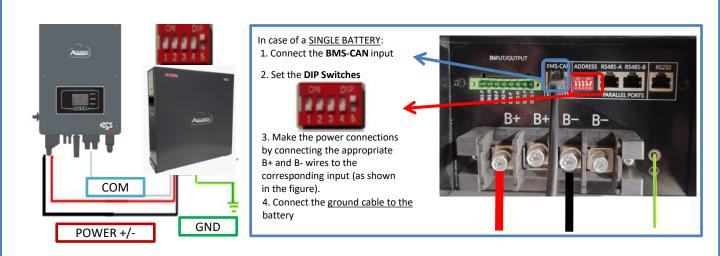
In case of <u>MULTIPLE BATTERIES</u>, connect the communication cable from the **CAN** port of the inverter to the **BMS-CAN** port of the MASTER battery, after having defined the correct positioning of the <u>DIP Switches</u> (see following pages).
