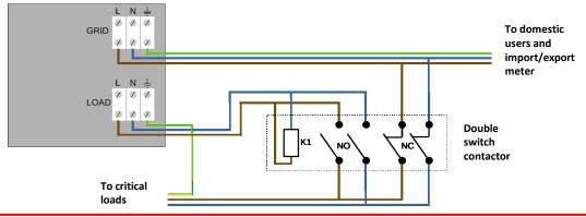
**NOTE:** For the conditions described above, in the event of a power failure, the part of the system powered by the inverter's LOAD port behaves like an IT system
