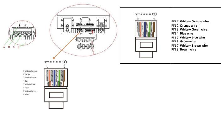
a) Logic interface for AS/NZS 4777.2:2015, also known as inverter demand response modes (DRMs). The inverter will detect and initiate a response to all supported demand response commands within 2s. The inverter will continue to respond while the mode remains asserted.
