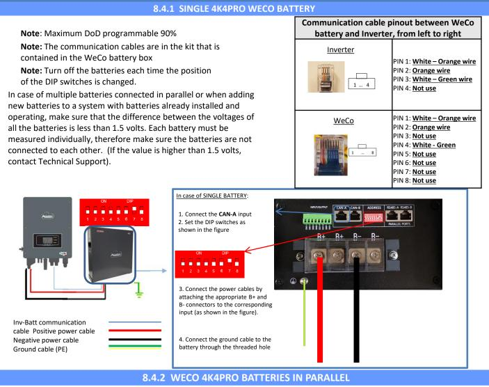
In case of <u>MULTIPLE BATTERIES</u>, connect the communication cable from the CAN port of the inverter to the CAN- A port of the MASTER battery after defining the correct positioning of the DIP switches:
