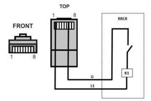
Here below the <u>function description of the terminal</u>. **Relay status**: close is 1, open is 0.
