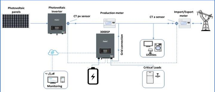
The wiring diagram for the 3000SP single-phase storage system is shown above. For instructions on this installation mode, refer to all pages of this guide, except pages 16 to 22 (inclusive).
