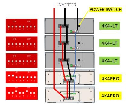
Communication connections between batteries and inverter: Batteries are connected IN PARALLEL to each other.
