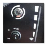
2. Inverter DC rotary switch set to OFF;
