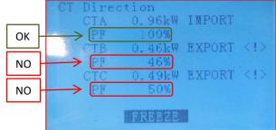
Block the CTs by pressing the arrow for the word **FREEZE** appears at the bottom and then confirm with the fourth button
