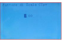
**NOTE**: The CTpv scale factor is the multiplying coefficient of the power value read by the CTpv sensor on the phase in which it is installed.
