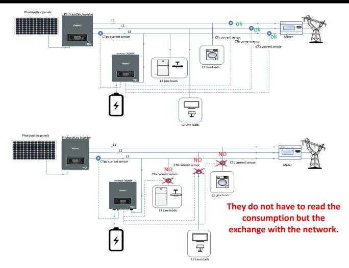
Each sensor must include all phase cables entering or exiting from the meter.
