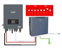
Inv-Batt communication cable Positive power cable Negative power cable Ground cable (PE)
