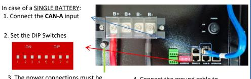
3. The power connections must be made by attaching the appropriate B+ and B- connectors to the corresponding input (as shown in the figure). 4. Connect the ground cable to the battery through the threaded hole
