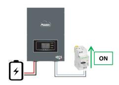
5) Check that the display shows a withdrawn power value equal to the absorbed power value which can be measured by placing a current clamp under the import/export meter.
