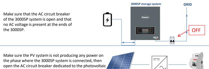
inverter to verify that no power is being produced.
