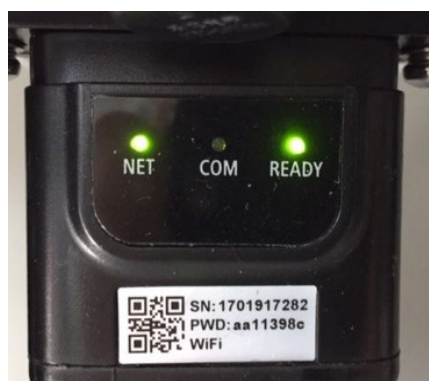
Figure 77- Irregular communication status between inverter and adapter
