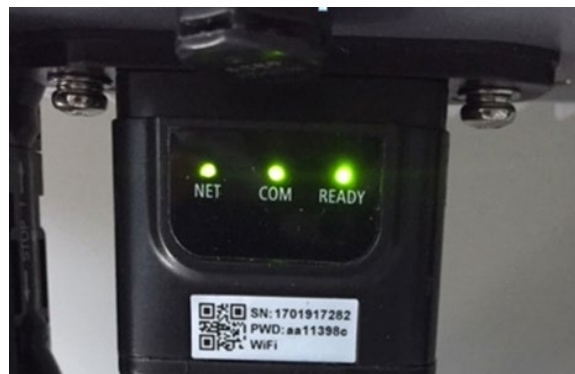
Figure 70 - Final status of LEDs
