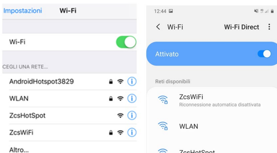
Figure 55 – Wi-Fi network search on Smartphone (iOS and Android); Access point of the Wi-Fi adapter is no longer visible
