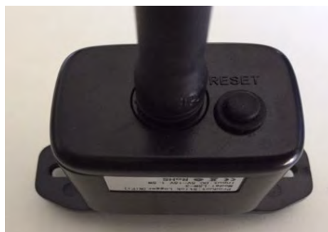
Figure 78 – Reset button on the Wi-Fi adapter
