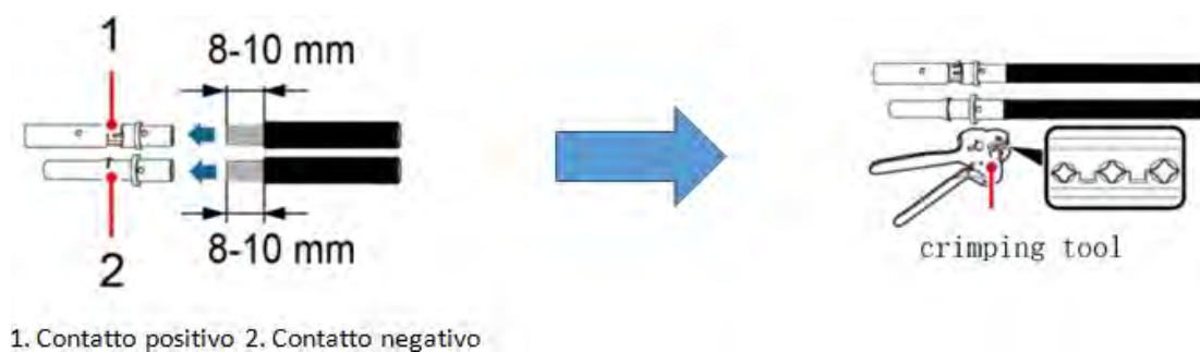
Figure 32 - Preparing the positive and negative photovoltaic cables
