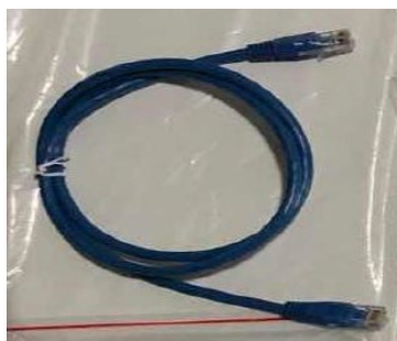
Figure 28 - Communication cable between WeCo 5k3 batteries
