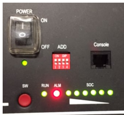
Figure 69 – Battery status after setting the POWER switch to ON and pressing the SW button
