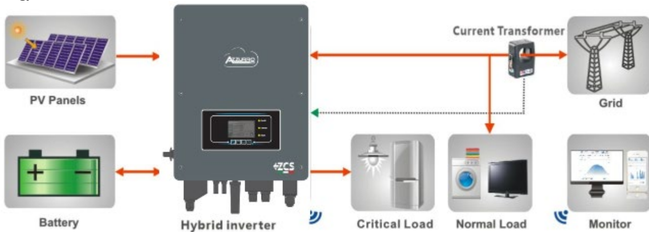
Figure 1 - Diagram of a system on which an 1PH HYD3000-HYD6000-ZSS hybrid is installed
