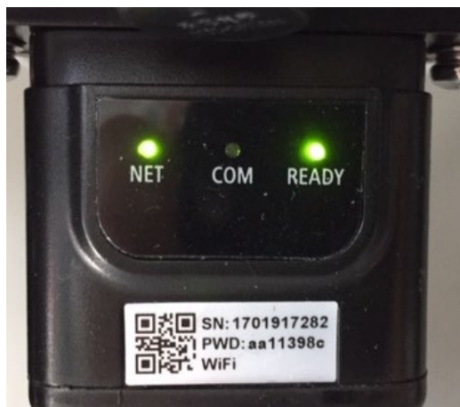
Figure 104 - Irregular communication status between the inverter and adapter
