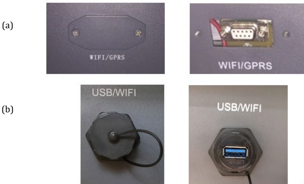
Figure 73 – Port for external Wi-Fi adapter
