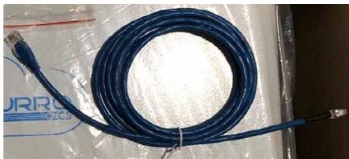
Figure 33 - Communication cable between the inverter and WeCo 5K3XP battery
