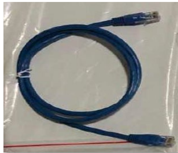
Figure 48 – Communication cable between AZZURRO 5000 PRO batteries
