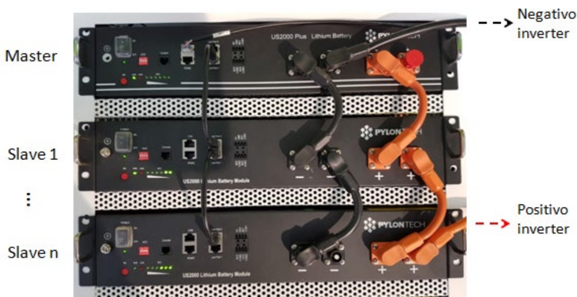
Figure 10 – Connecting three Pylontech batteries in parallel
