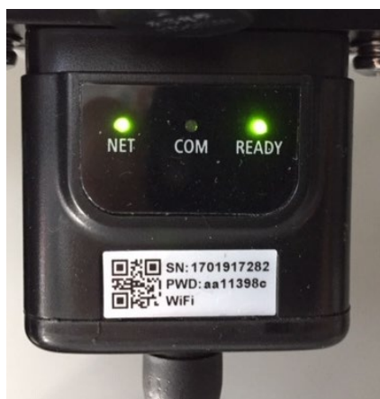
Figure 93 - Irregular communication status between inverter and Wi-Fi
