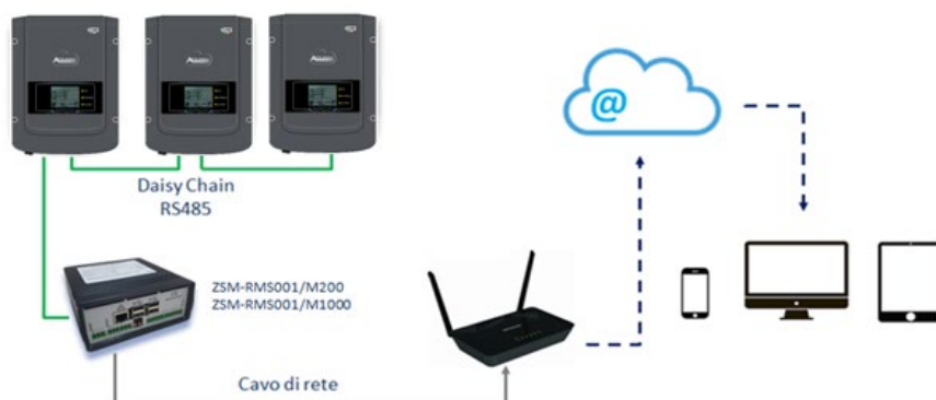
Figure 113 – Diagram showing the operation of the ZSM-RMS001/M200 / ZSM-RMS001/M1000 datalogger
