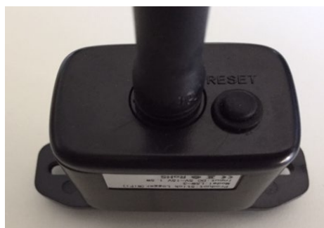
Figure 92 – Reset button on the Wi-Fi adapter
