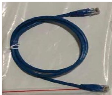
Figure 21 – Communication cable between WeCo 4k4 PRO batteries
