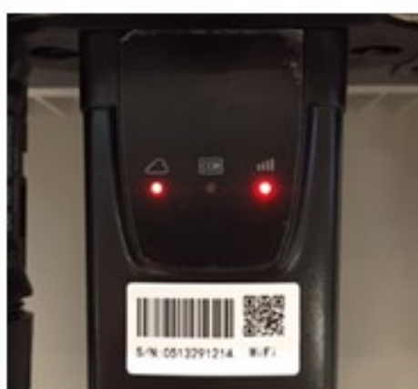
Figure 93 - Irregular communication status between inverter and Wi-Fi
