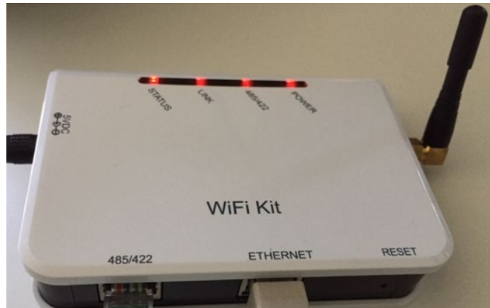
Figure 133 – LED indicating the correct configuration of the datalogger
