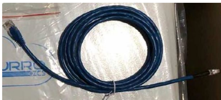
Figure 44 - Communication cable between the inverter and AZZURRO 5000 PRO battery
