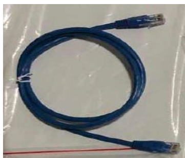
Figure 48 – Communication cable between AZZURRO 5000 batteries
