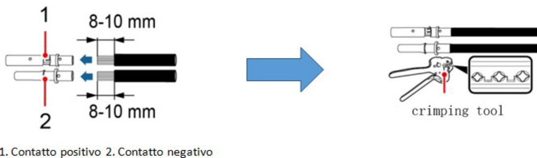
Figure 52 – Preparing the positive and negative photovoltaic cables
