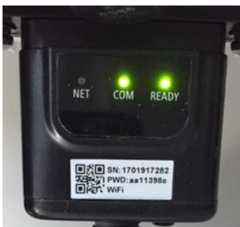
Figure 95 - Irregular communication status between Wi-Fi and remote server
