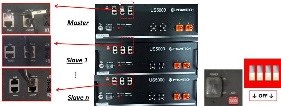
Figure 14 - Connecting the communication cable between three Pylontech batteries
