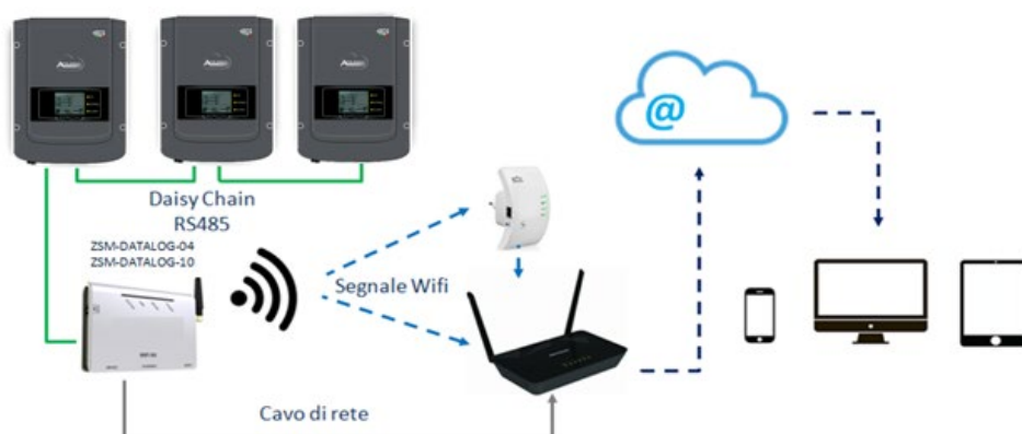
Figure 112 – Diagram for connecting the ZSM-DATALOG-04 / ZSM-DATALOG-10 datalogger
