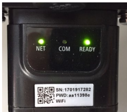
Figure 110 - Irregular communication status between inverter and adapter
