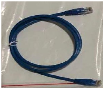
Figure 48 – Câble de communication entre batteries AZZURRO 5000 PRO
