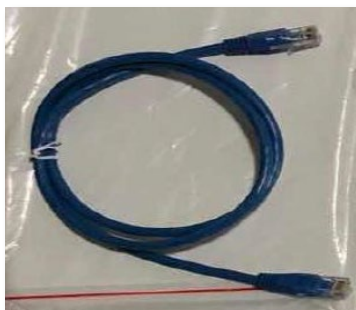
Figure 51 – Câble de communication entre batteries AZZURRO ZSX 5000 S
