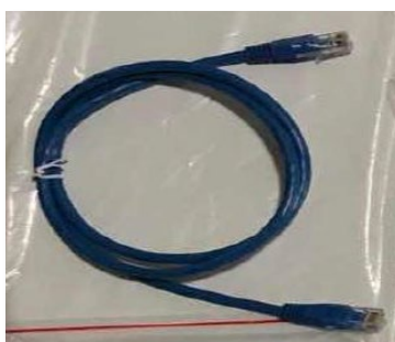
Figure 6 – Câble de communication entre batteries WeCo 4k4-LT
