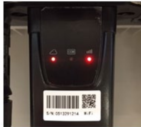
Figure 123 - Irregular communication status between inverter and Wi-Fi
