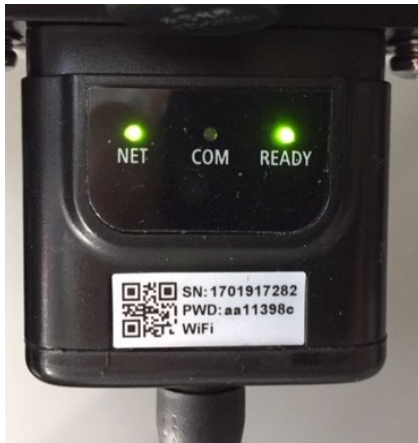
Figure 123 - Irregular communication status between inverter and Wi-Fi
