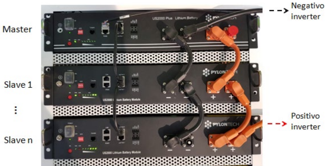
Figure 15 - Connecting three Pylontech batteries in parallel
