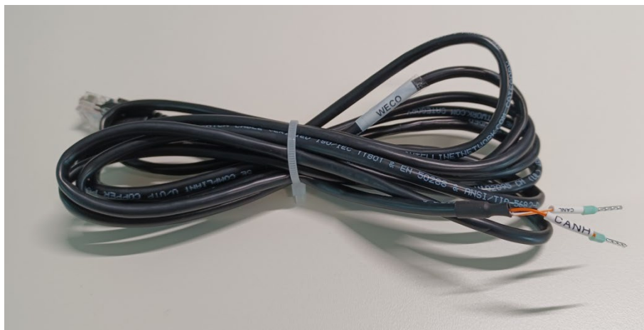
Figure 37 - Communication cable between the inverter and WeCo 4k4-LT battery
