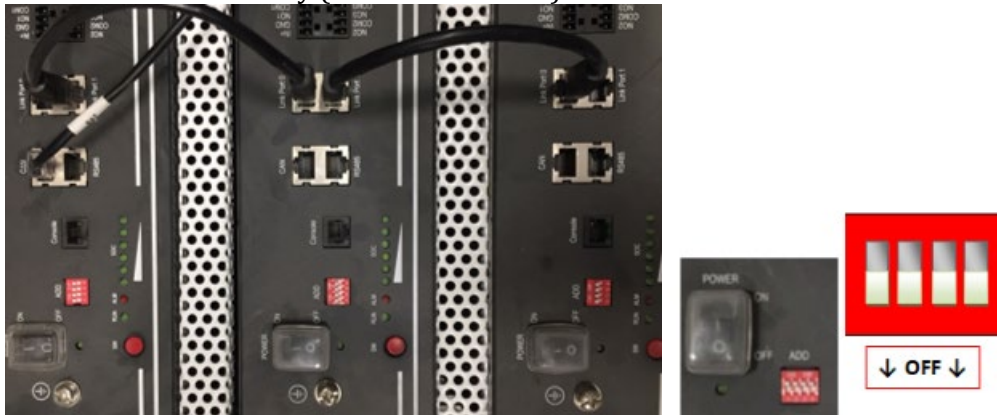
Figure 14- Connecting the communication cable between three Pylontech batteries
