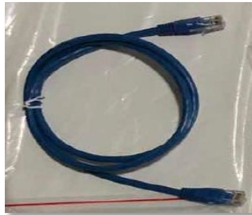
Figure 48 – Communication cable between WeCo 5k3 batteries
