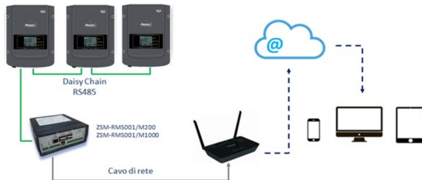
Figure 143 – Diagram for the functioning of the ZSM-RMS001/ M200 / ZSM-RMS001/M1000 datalogger
