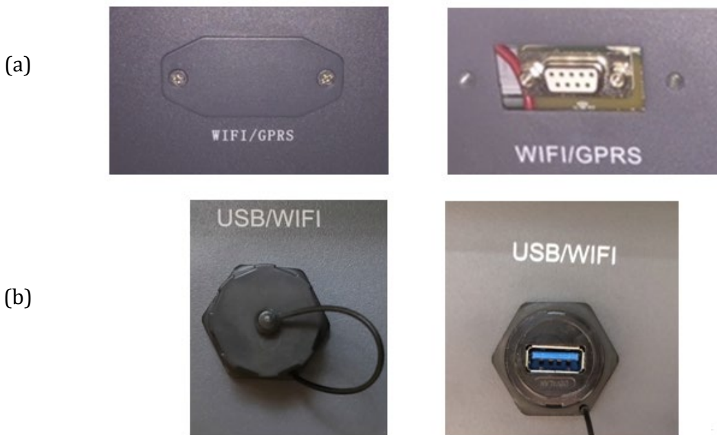
Figure 104 - Slot for external Wi-Fi adapter
