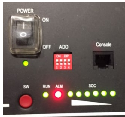
Figure 101 - Battery status after setting the POWER switch to ON and pressing the SW button
