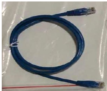
Figure 77 – Communication cable between AZZURRO 5000 PRO batteries
