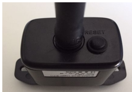
Figure 122 – Reset button on the Wi-Fi adapter
