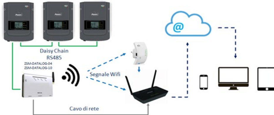
Figure 142 – Diagram for connecting the ZSM-DATALOG-04 / ZSM-DATALOG-10 datalogger
