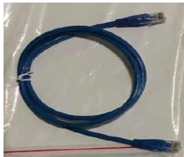
Figure 32 – Communication cable between WeCo 4k4 PRO batteries
