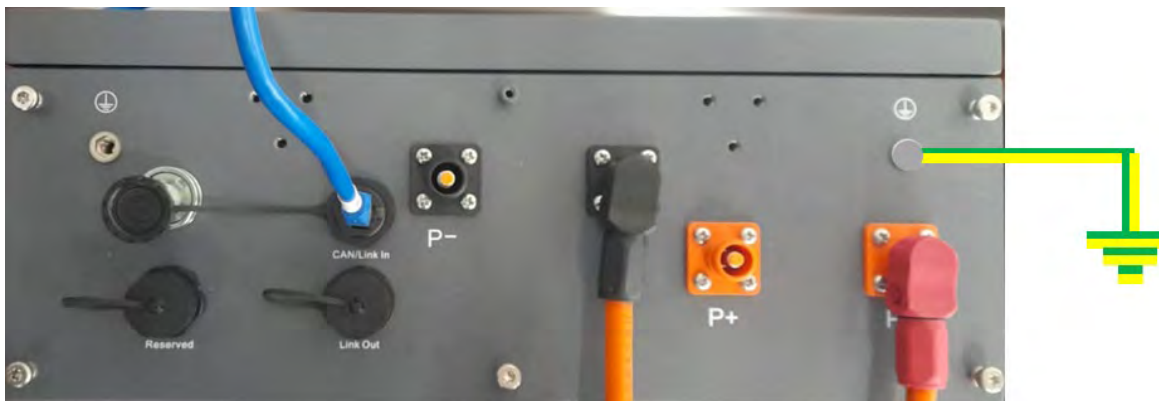
Figure 94 – Terminal block of the AZZURRO 5000S battery
