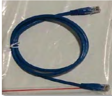
Figure 96 – Communication cable between AZZURRO 5000S batteries
