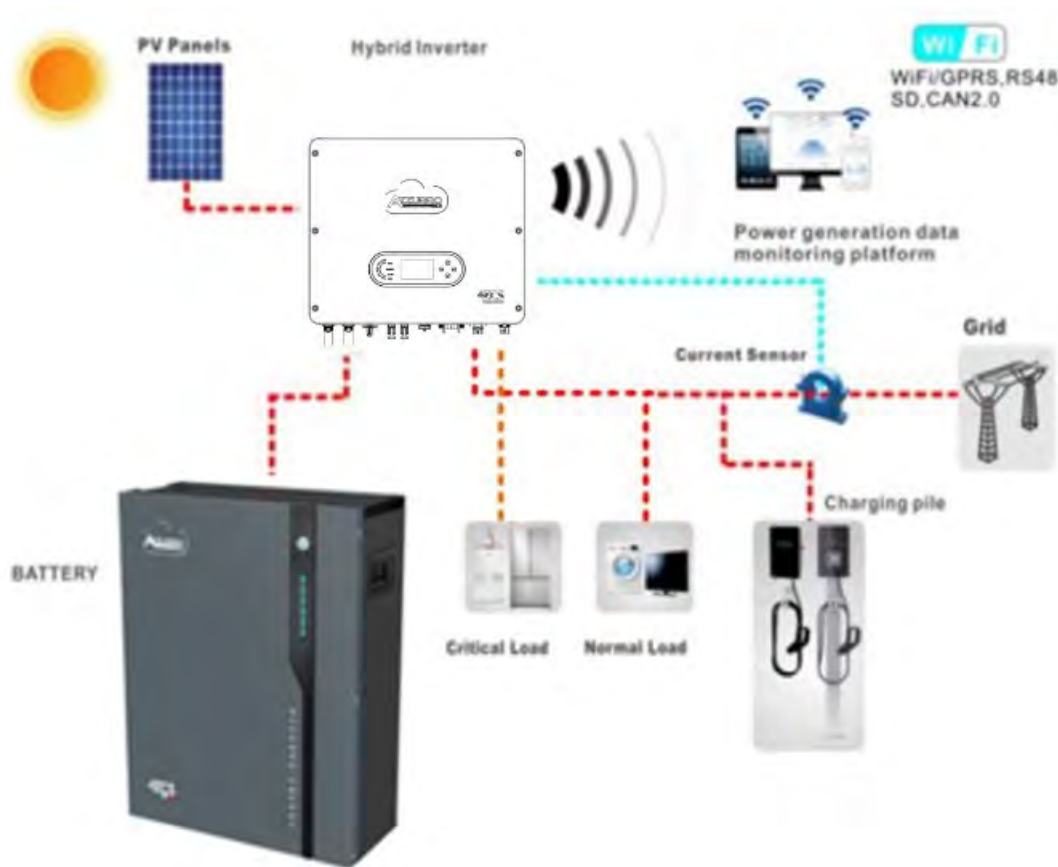
Figure 1 - Diagram of a system on which an 1PH HYD3000-HYD6000-ZSS-HP hybrid inverter is installed
