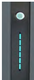
Figure 78- Power button of the AZZURRO 5000 PRO battery
