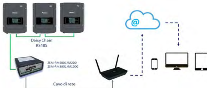
Figure 154 – Diagram for the functioning of the ZSM-RMS001/ M200 / ZSM-RMS001/M1000 datalogger
