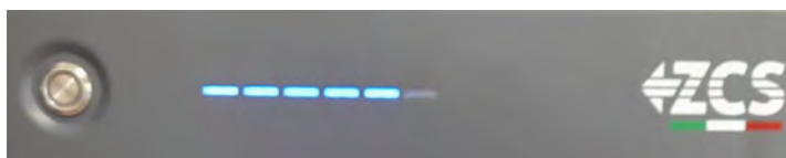
Figure 95– Power button of the AZZURRO 5000S battery
