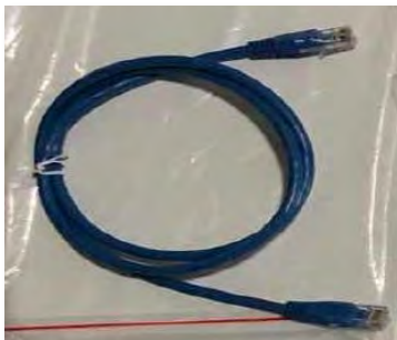
Figure 26 – Communication cable between WeCo 4k4 batteries
