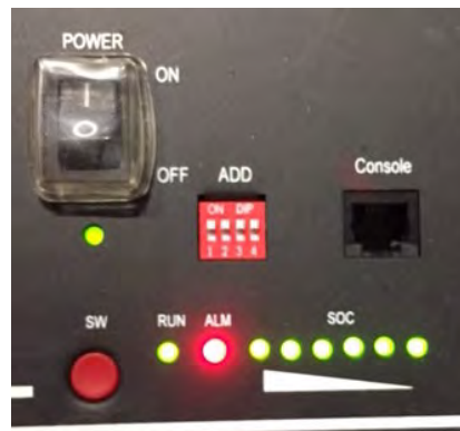
Figure 112 – Battery status after setting the POWER switch to ON and pressing the SW button
