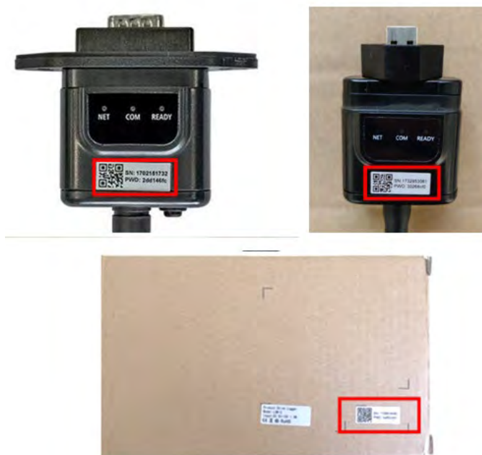
Figure 120 – Password of external Wi-Fi adapter
