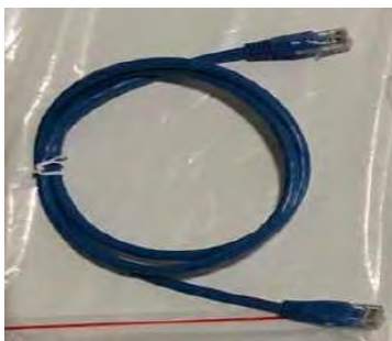
Figure 71 – Communication cable between AZZURRO 5000 batteries
