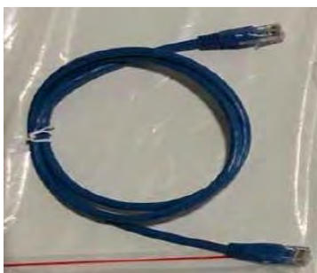
Figure 87 – Communication cable between AZZURRO ZSX 5120 batteries
