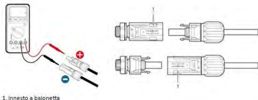
Figure 11 – Connecting the photovoltaic connectors
