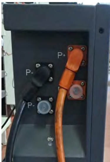
Figure 85 – Terminal block of the AZZURRO ZSX 5120 battery
