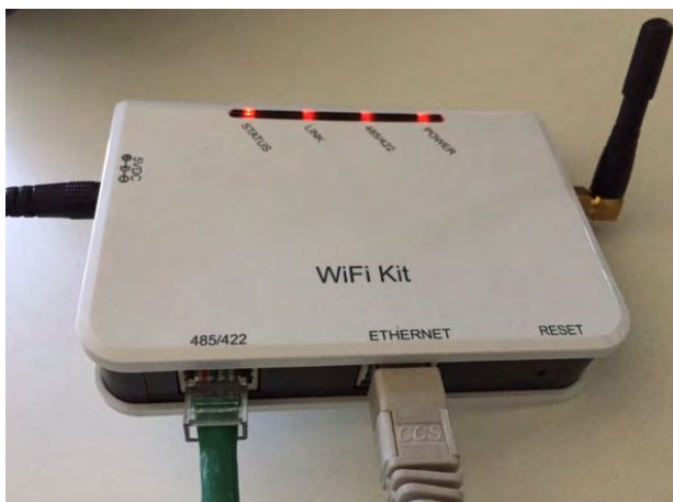
Figure 163 – Ethernet cable connected to the datalogger
