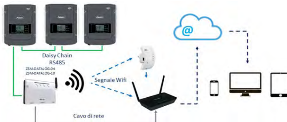
Figure 153 – Diagram for connecting the ZSM-DATALOG-04 / ZSM-DATALOG-10 datalogger
