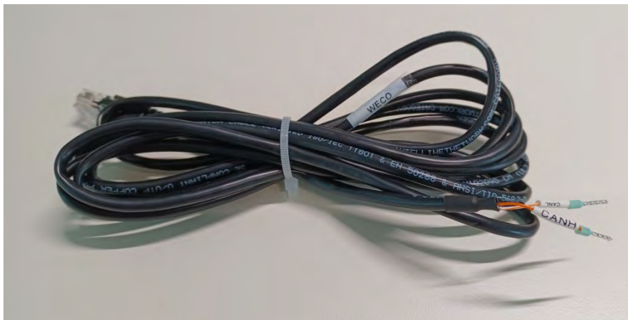
Figure 31 - Communication cable between the inverter and WeCo 4k4 PRO battery
