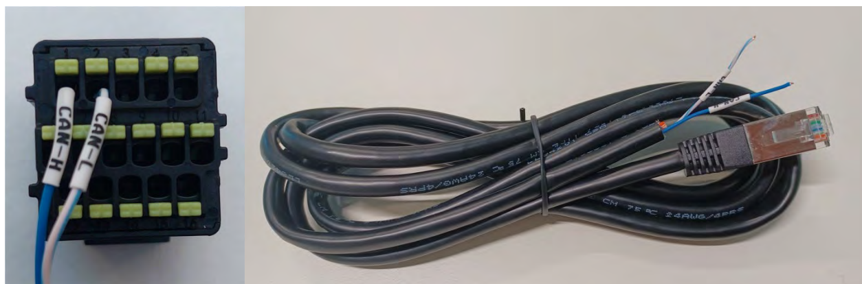
Figure 92 - Communication cable between the inverter and AZZURRO 5000S battery
