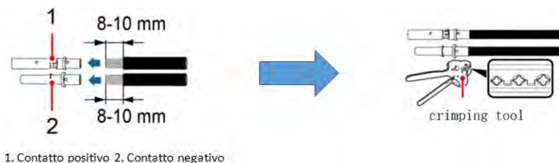
Figure 9 – Preparing the positive and negative PV cables
