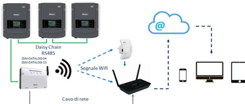
Figure 128 – Diagram for connecting the ZSM-DATALOG-04 / ZSM-DATALOG-10 datalogger
