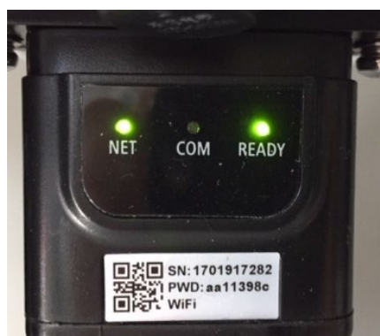
Figure 126 - Irregular communication status between inverter and adapter
