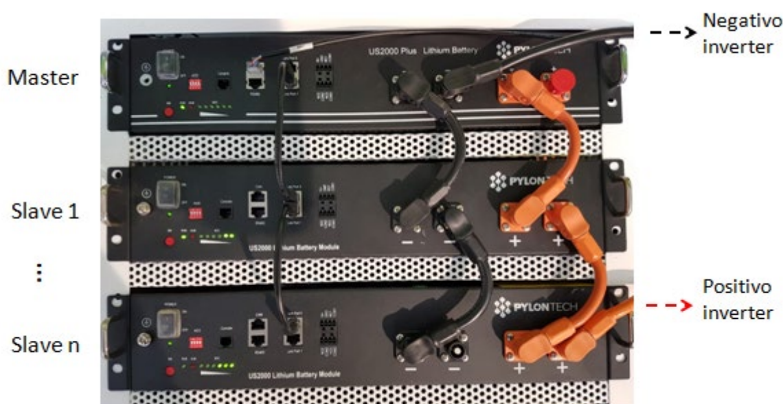
Figure 11 – Connecting three Pylontech batteries in parallel
