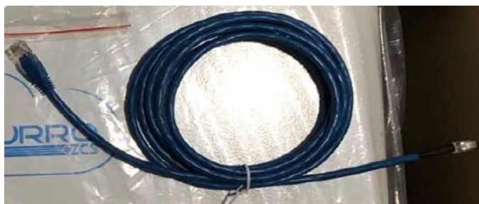
Figure 47 - Communication cable between the inverter and AZZURRO 5000 battery
