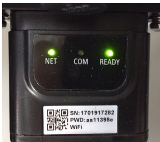
Figure 120 - Irregular communication status between the inverter and adapter
