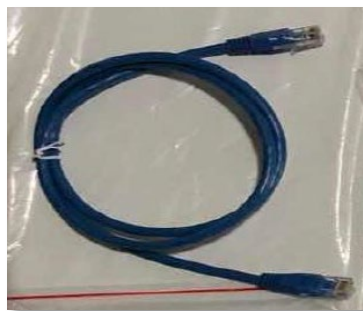
Figure 51 – Communication cable between AZZURRO 5000 batteries
