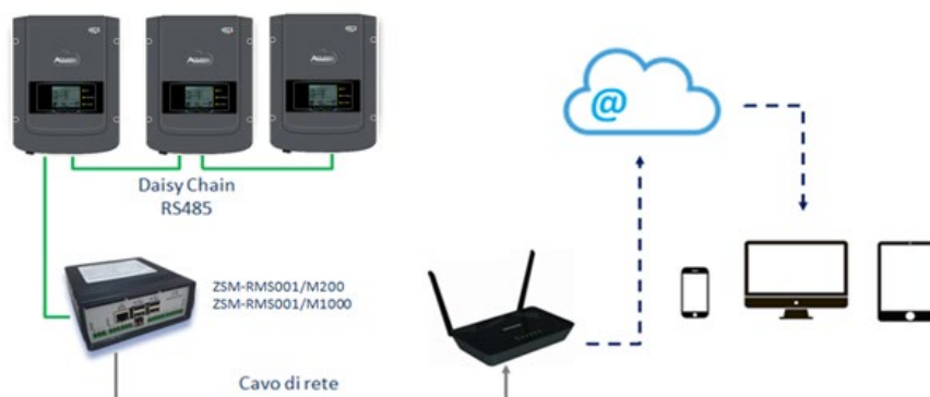
Figure 129 – Diagram showing the operation of the ZSM-RMS001/M200 / ZSM-RMS001/M1000 datalogger
