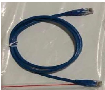
Figure 51 – Communication cable between AZZURRO ZSX 5120 batteries
