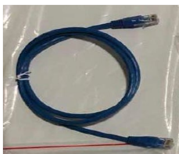
Figure 31 - Communication cable between WeCo 5k3 batteries
