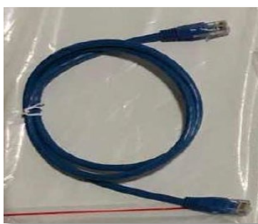
Figure 51 – Communication cable between AZZURRO 5000 batteries
