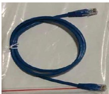
Figure 24 – Communication cable between WeCo 4k4 LT batteries
