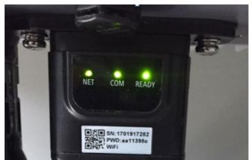
**Figure 56 - Final status of LEDs**
