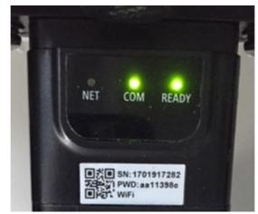
Figure 58 - Irregular communication status between the adapter and remote server
