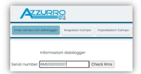
Enter the serial number (S/N) of the datalogger and click "Check RMS". If the datalogger has been configured correctly, a screen will open where you can enter the required information relating to the field to be installed.
