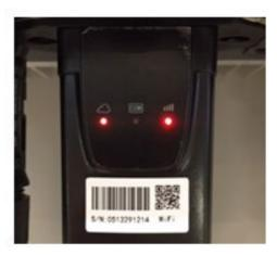
Figure 46 - Irregular communication status between inverter and Wi-Fi
