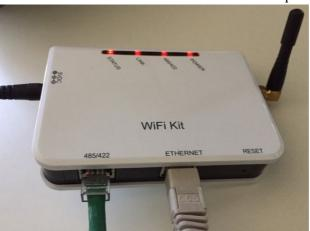
Figure 83 - Ethernet cable connected to the datalogger
