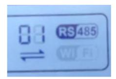
Figure 82 - RS485 symbol on the display of the inverter
