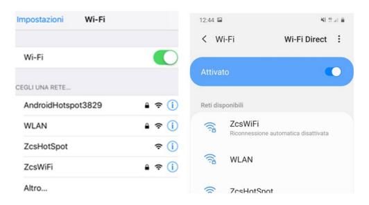
Figure 41 - Wi-Fi network search on Smartphone (iOS and Android); Access point of the Wi-Fi adapter is no longer visible
