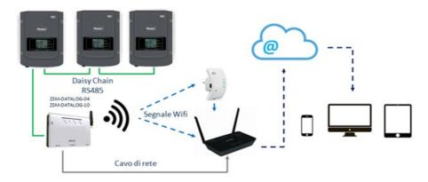
Figure 65 - Diagram for connecting the ZSM-DATALOG-04 / ZSM-DATALOG-10 datalogger
