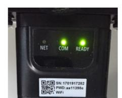
Figure 64 - Irregular communication status between the adapter and remote server
