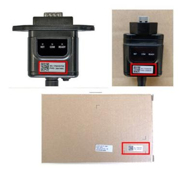
Figure 31 - Password of external Wi-Fi adapter
