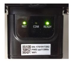
Figure 63 - Irregular communication status between inverter and adapter
