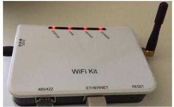
Figure 95 - LED indicating the correct configuration of the datalogger
