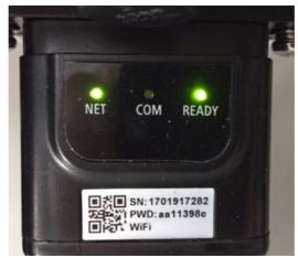
Figure 57 - Irregular communication status between the inverter and adapter
