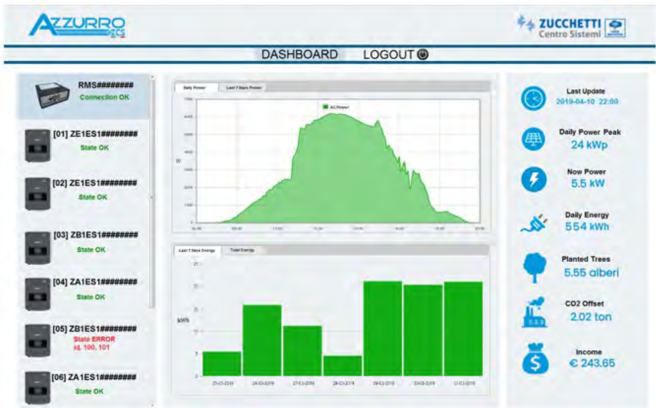
Figure 99 – Example of local monitoring page
