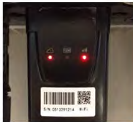
Figure 53 – Irregular communication status between inverter and Wi-Fi
