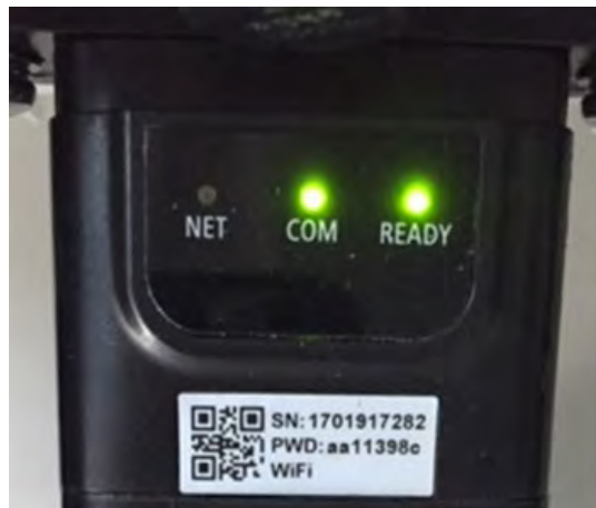
Figure 65 – Irregular communication status between the adapter and remote server
