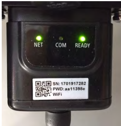
Figure 53 – Irregular communication status between inverter and Wi-Fi
