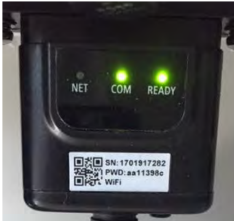
Figure 55 - Irregular communication status between Wi-Fi and remote server
