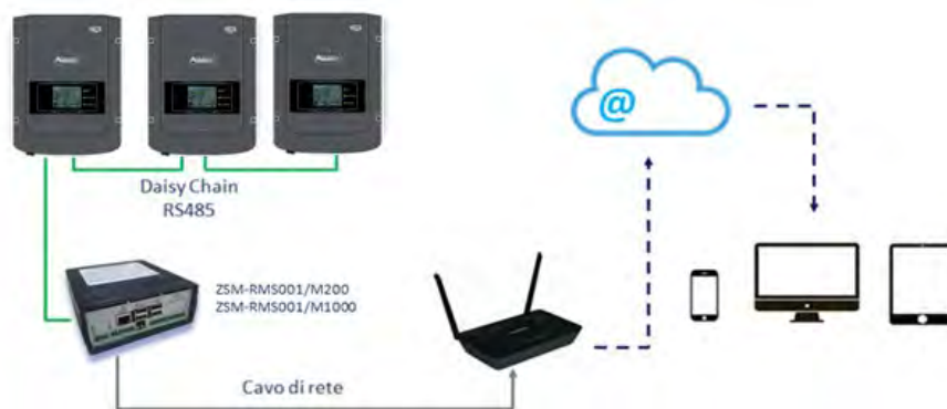
Figure 73 – Diagram showing the operation of the ZSM-RMS001/M200 / ZSM-RMS001/M1000 datalogger
