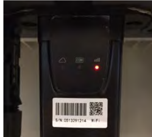
Figure 55 - Irregular communication status between Wi-Fi and remote server
