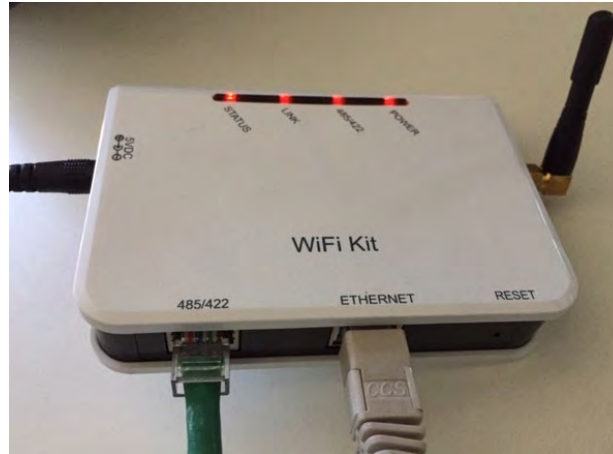
Figure 82 – Ethernet cable connected to the datalogger
