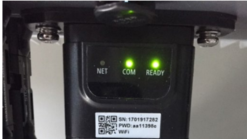
Figure 71 - Initial status of LEDs
