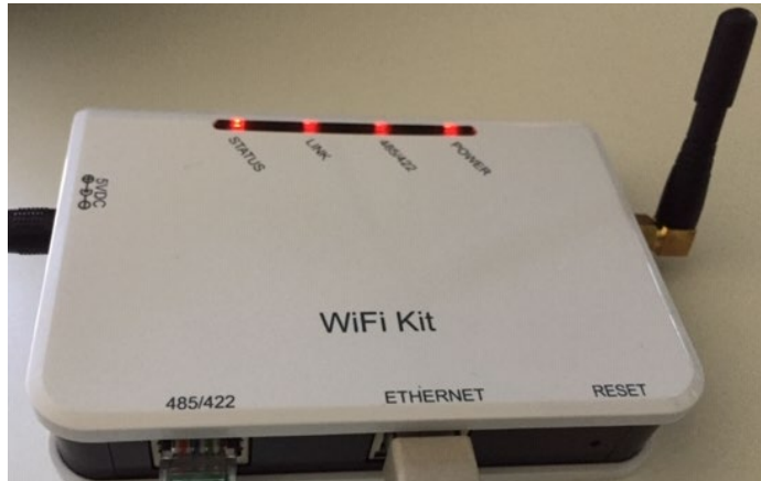
Figure 102 - LED indicating the correct configuration of the datalogger
