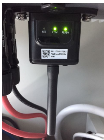
Figure 59 - Initial status of LEDs
