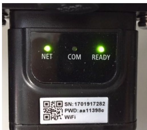
Figure 73 - Irregular communication status between the inverter and adapter
