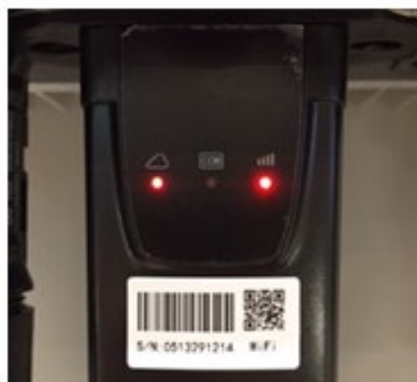
Figure 62 - Irregular communication status between inverter and Wi-Fi
