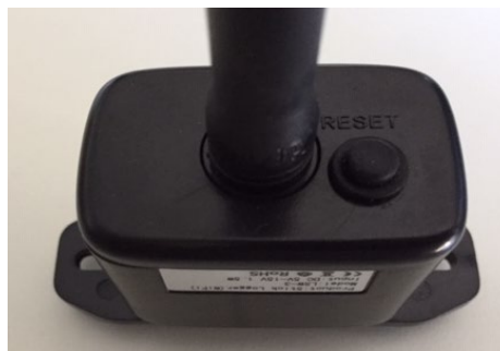
Figure 61 – Reset button on the Wi-Fi adapter
