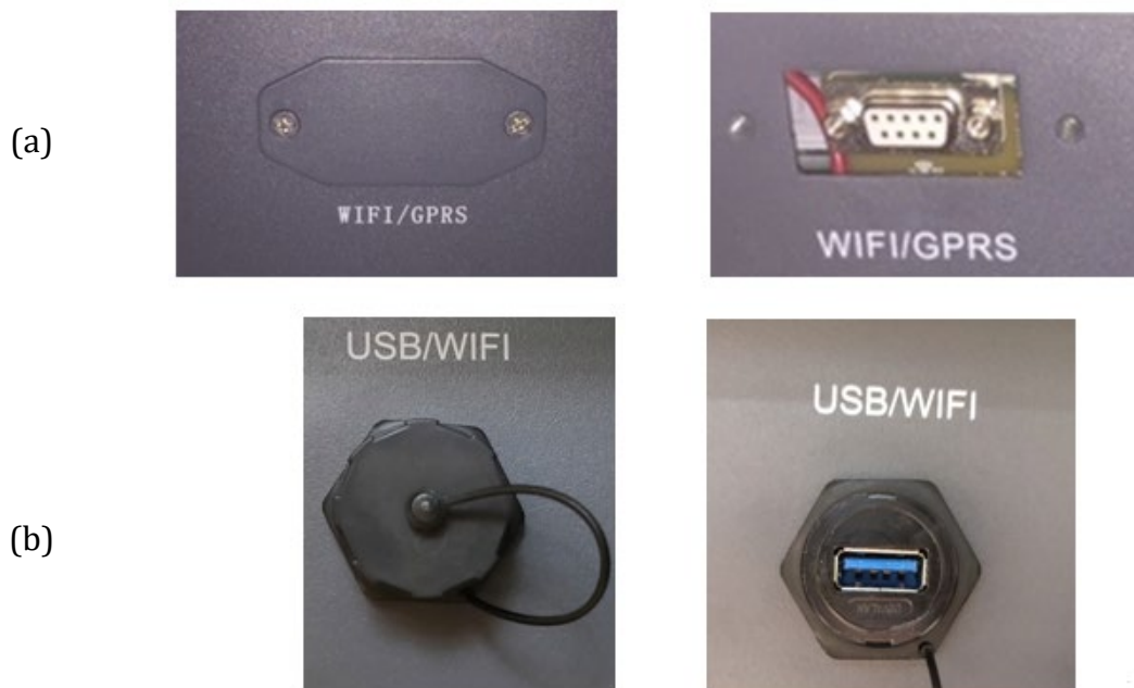
Figure 42 – Port for external Wi-Fi adapter
