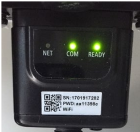
Figure 64 - Irregular communication status between Wi-Fi and remote server
