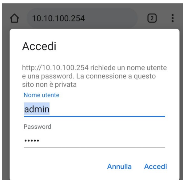
Figure 94 - Screen for logging into the web server to configure the datalogger
