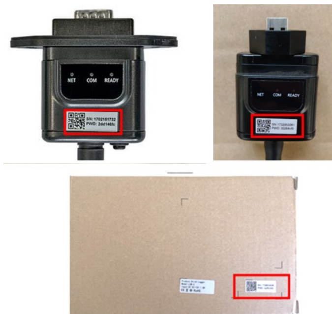
Figure 47 - Password of external Wi-Fi adapter
