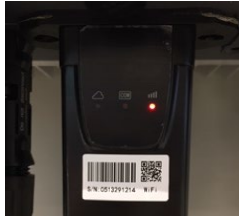
Figure 64 - Irregular communication status between Wi-Fi and remote server
