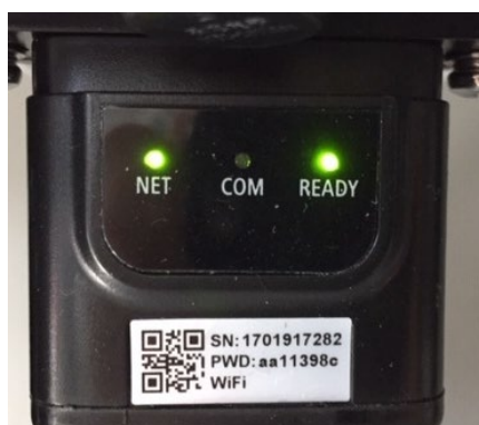
Figure 79 - Irregular communication status between inverter and adapter
