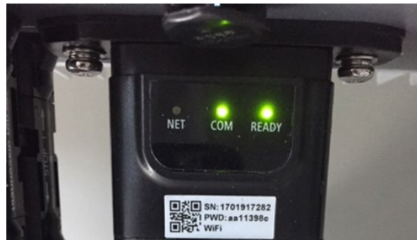
Figure 77 - Initial status of LEDs
