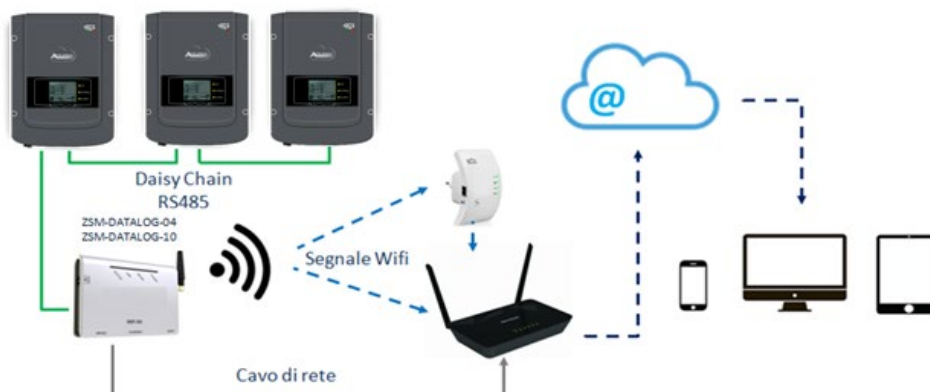
Figure 81 – Diagram for connecting the ZSM-DATALOG-04 / ZSM-DATALOG-10 datalogger
