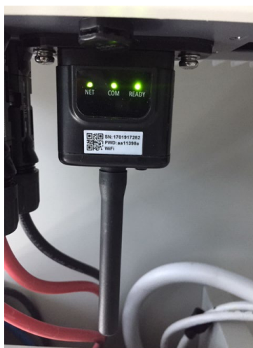
Figure 60 - Final status of LEDs
