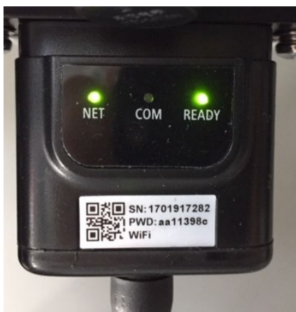
Figure 62 - Irregular communication status between inverter and Wi-Fi
