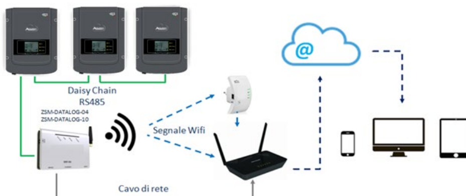
Figure 81 – Diagram for connecting the ZSM-DATALOG-04 / ZSM-DATALOG-10 datalogger
