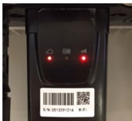
Figure 62 - Irregular communication status between inverter and Wi-Fi
