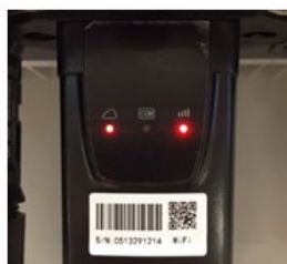
Figure 5-52 - Irregular communication status between inverter and Wi-Fi
