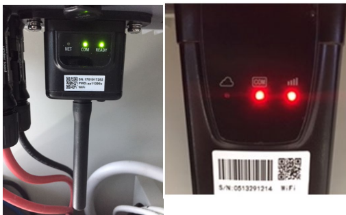
Figure 5-51 - Initial status of LEDs
