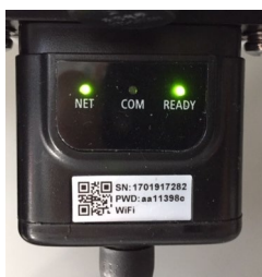
Figure 5-52 - Irregular communication status between inverter and Wi-Fi
