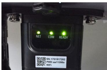
Figure 5-59 - Final status of LEDs
