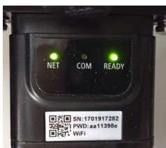
Figure 5-59 - Irregular communication status between the inverter and adapter
