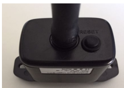
Figure 5-52 - Reset button on the Wi-Fi adapter
