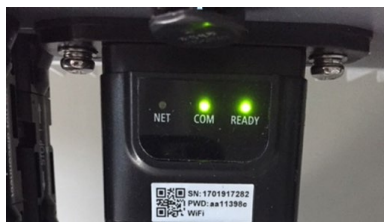
Figure 5-61 - Initial status of LEDs
