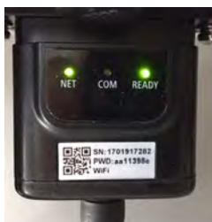
Figure 5-52 - Irregular communication status between inverter and Wi-Fi
