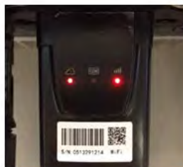
Figure 5-52 - Irregular communication status between inverter and Wi-Fi
