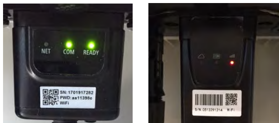
Figure 5-54 - Irregular communication status between Wi-Fi and remote server
