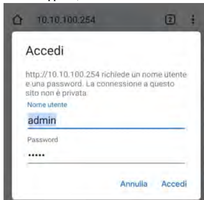
Figure 5-44 – Screen for accessing the web server to configure the Wi-Fi adapter
