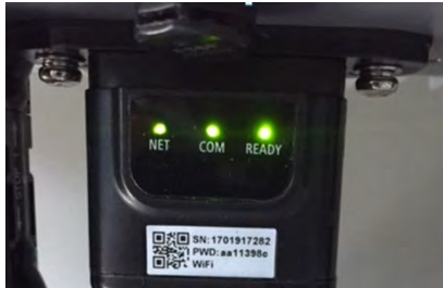
Figure 5-62 - Final status of LEDs
