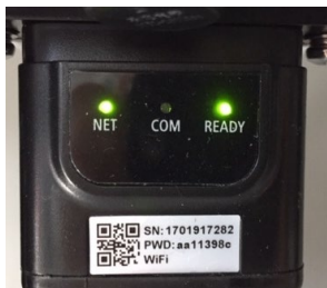
Figure 5-62 - Irregular communication status between inverter and adapter
