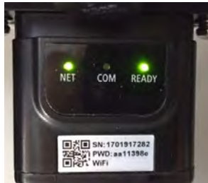
Figure 5-62 - Irregular communication status between inverter and adapter
