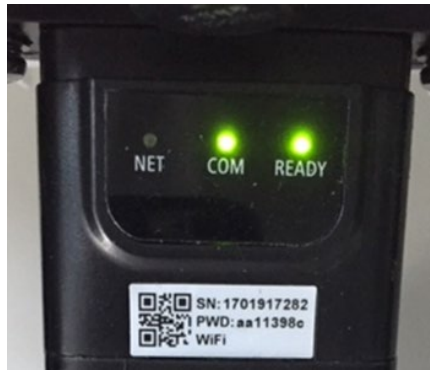
Figure 110 - Irregular communication status between the adapter and remote server
