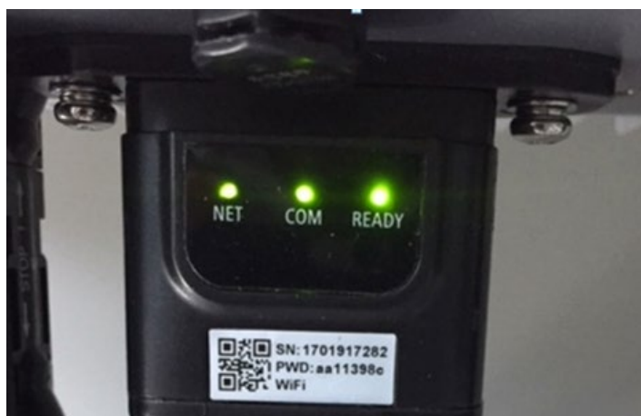
Figure 102 - Final status of LEDs
