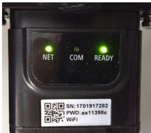
Figure 103 - Irregular communication status between the inverter and adapter
