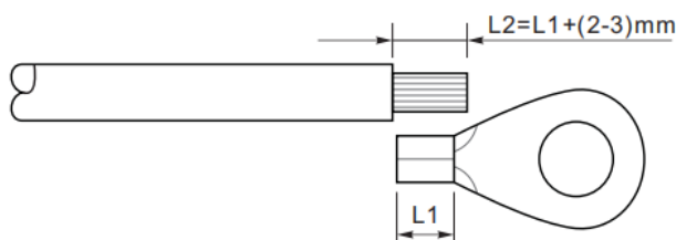
Figure 11 - Removal of insulating layer
