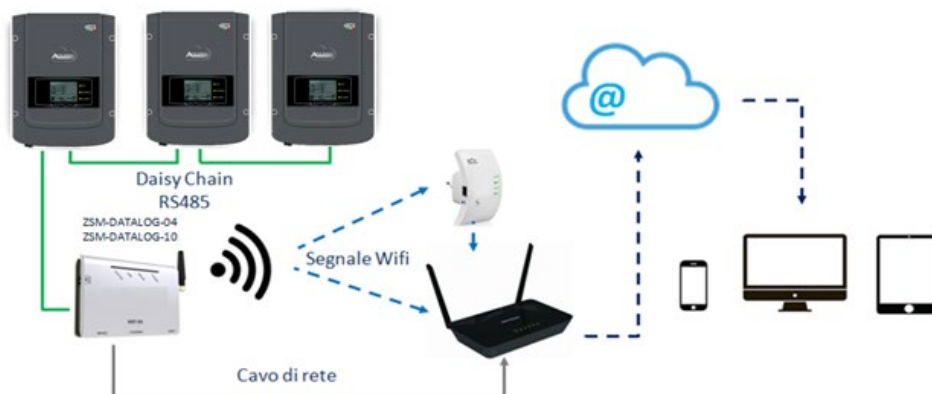
Figure 217 – Diagram for connecting the ZSM-DATALOG-04 / ZSM-DATALOG-10 datalogger
