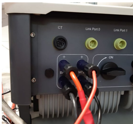
Figure 64 - Inverter-side DC power connection with two battery inputs populated
