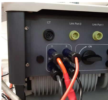
Figure 111 - Inverter-side DC power connection with two battery inputs populated
