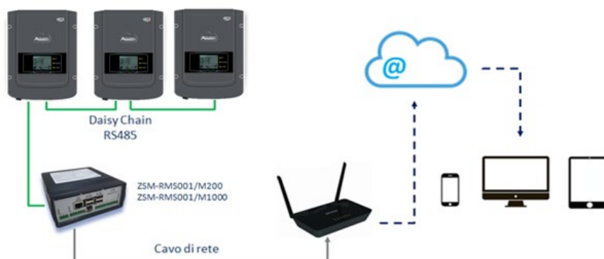
Figure 218 – Diagram for the functioning of the ZSM-RMS001/ M200 / ZSM-RMS001/M1000 datalogger
