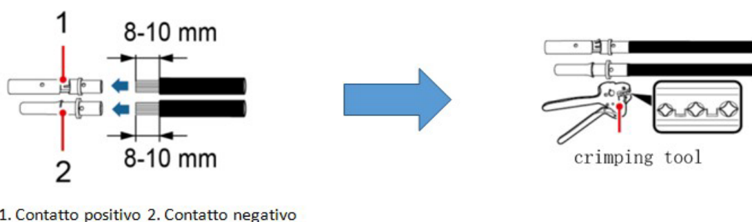
Figure 20 – Preparing the positive and negative photovoltaic cables
