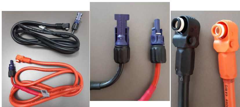
Figure 46 - BMS Inverter power cables (left), inverter-side power terminals (centre), battery-side power terminals (left)
