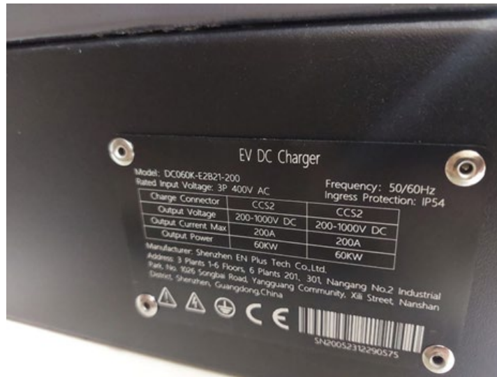
Figure 2 - Labels present on the charging station
