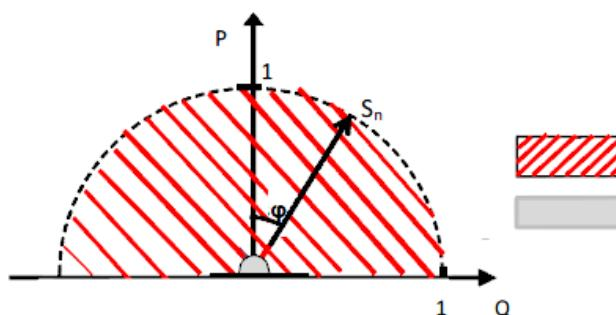
**Picture 16-Capability for static generators in power plants > 400 kW
