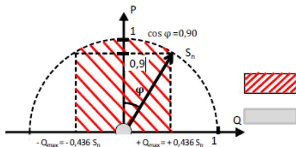
**Capability for static generators in power plants < 400 kW
